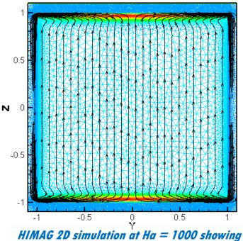
HIMAG 2D simulation at Ha = 1000 showing good accuracy and current conservation on triangular mesh
