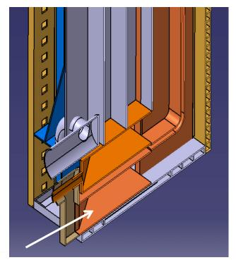
Manifold with feed from top instead of in-line
