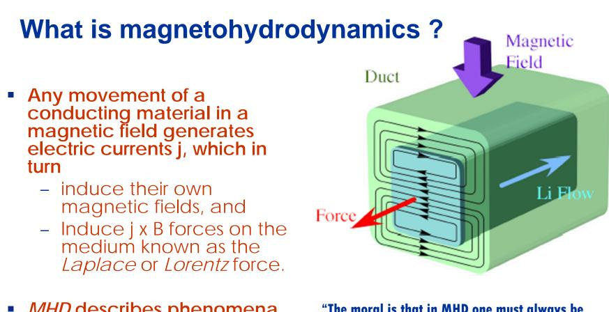
MHD describes phenomena in electrically conducting fluids, where the velocity field V, and the magnetic field B, are coupled. "The moral is that in MHD one must always be prepared to consider the complete electromagnetic field. The current and magnetic fluxes must have complete paths which may extend outside the region of fluid-mechanical interest into locations whose exact position may be crucial."
