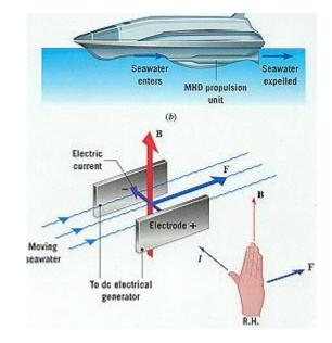
Generation of propulsion force by applying j and B in *Yamato 1* (Mitsubishi, 1991).
