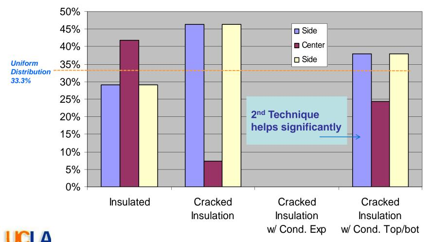
As predicted, the fast channels are pumping the slow channels by driving current that produces positive J x B force
