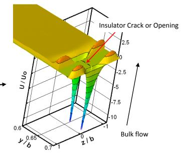
Reversed flow jets in region near cracks in insulator – Local reversed velocity 10x The average forward flow
